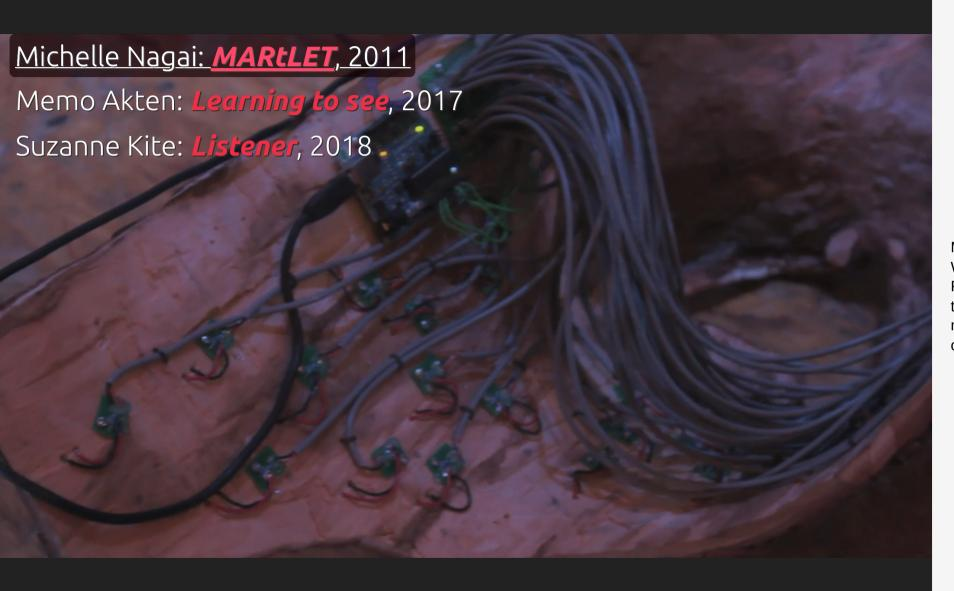
Michelle Nagai's *MARtLET* instrument uses the Wekinator software developed by Dr. Rebecca Fiebrink, to translate shadow and light into audio tones to create music. Wekinator allows artists to more easily associate sensor signals with particular outputs.
